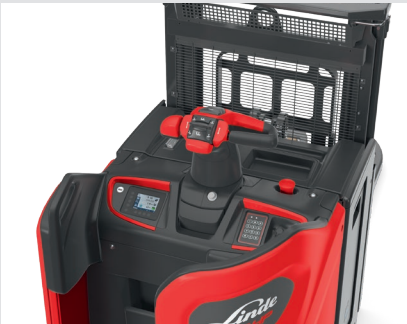
Ergonomic, height-adjustable tiller
